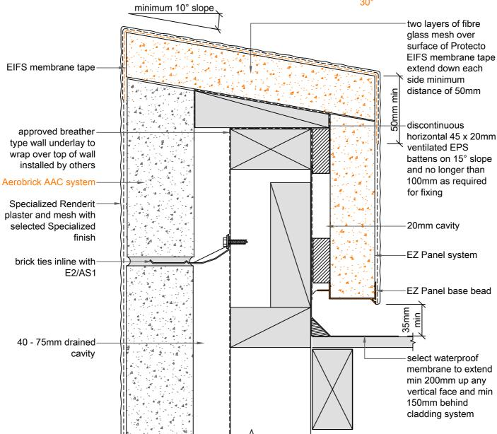
note: if roof is being used as an internal gutter the cladding must be a minimum of 100mm above the membrane surface
