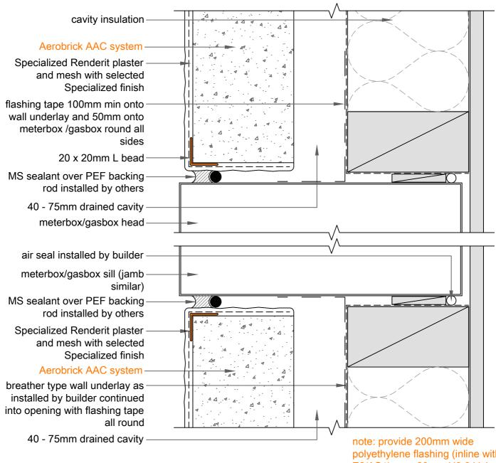
polyethylene flashing (inline with E2/AS1) over 20mm H3.2 kick out batten. sill flashing to extend 200mm past each end of meter box - by others
