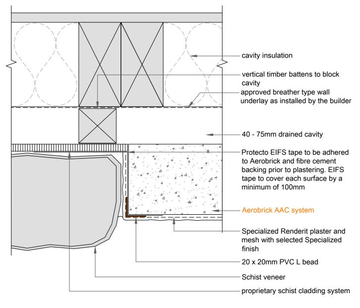
note: the Aerobrick AAC system must be installed and painted prior to schist being applied
