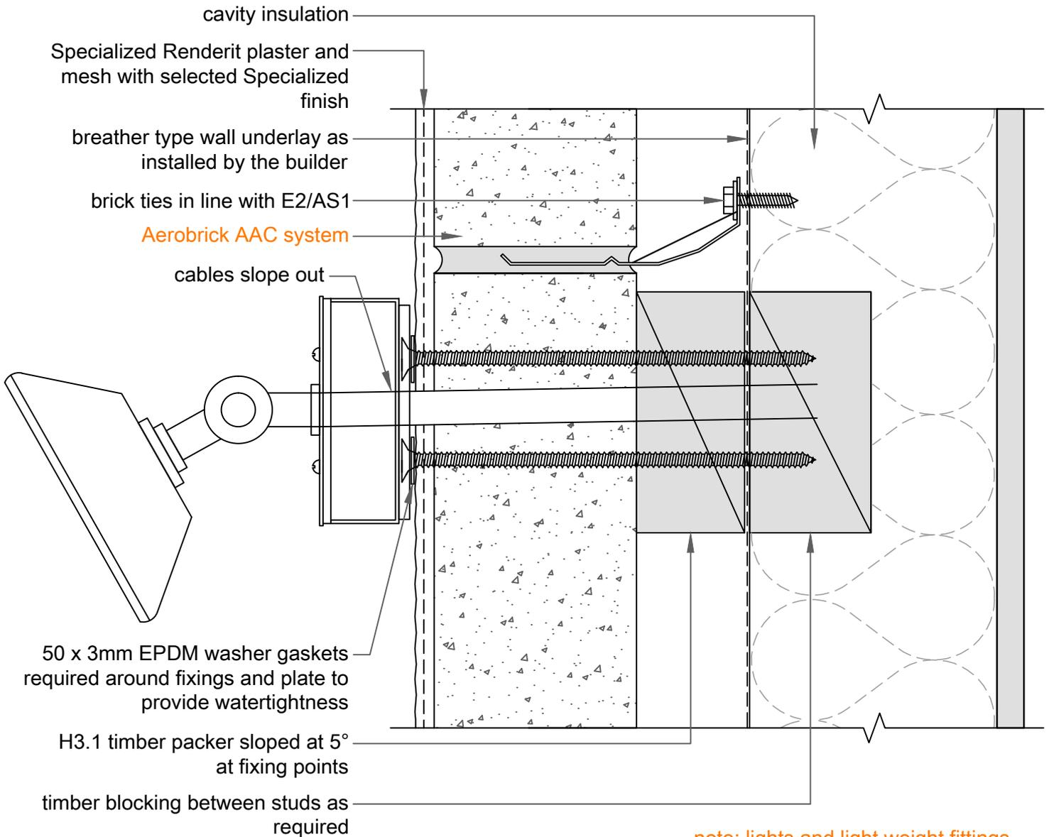
note: all electrical wiring should be enclosed in conduit
