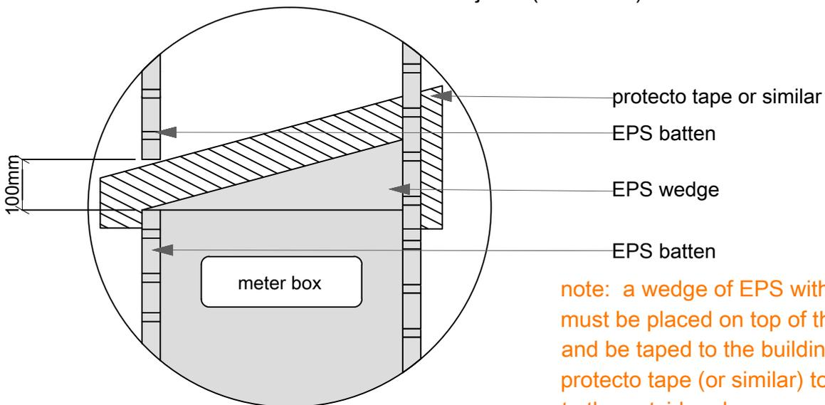
**note:** a wedge of EPS with a 15° slope must be placed on top of the meter box and be taped to the building wrap using protecto tape (or similar) to shed water to the outside edge. ensure tip of the wedge is not blocked by a vertical batten
