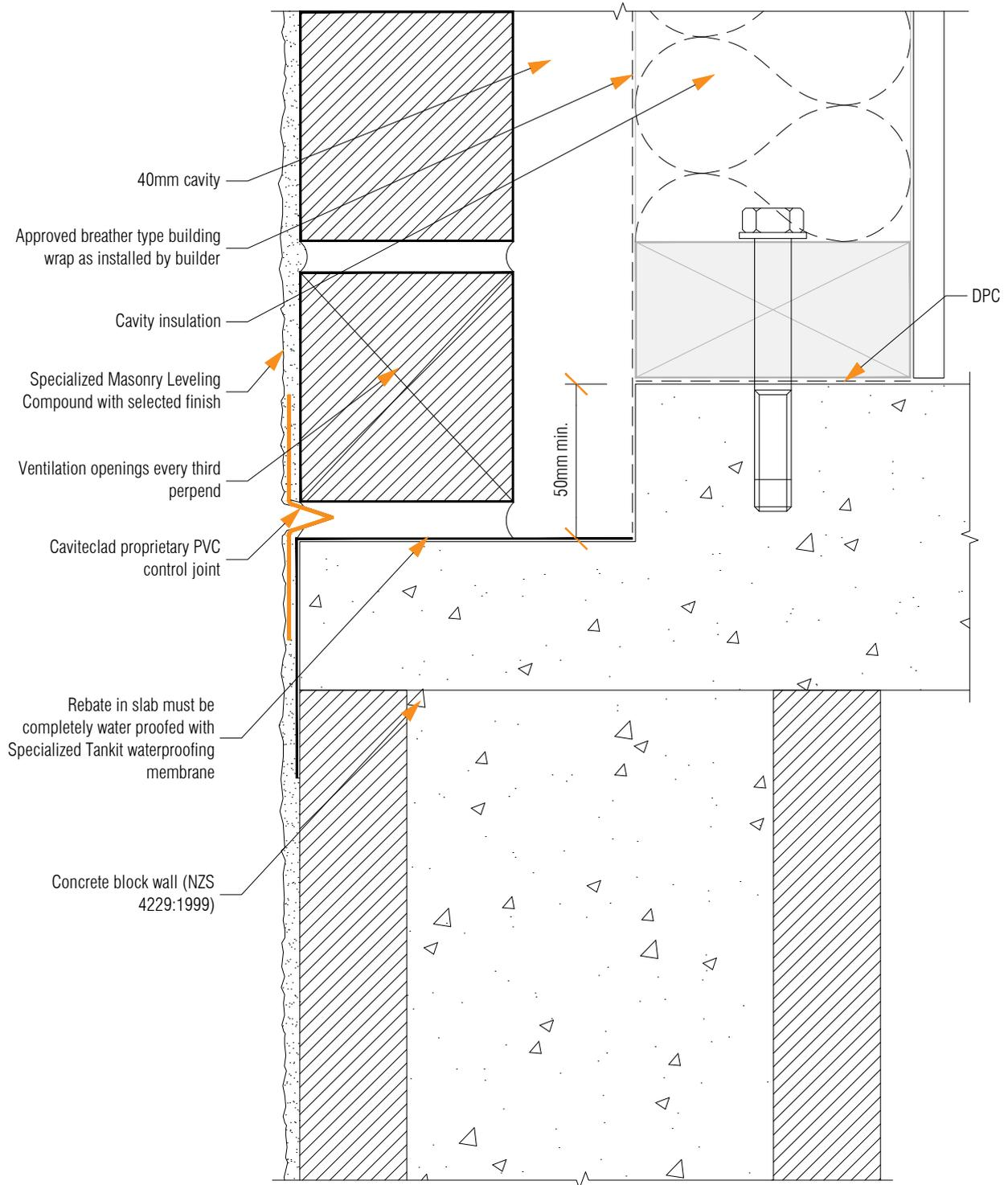
04 rebated concrete slab detail control joint.dwg
