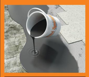
Pourite SLC is a one component polymer rich cementitious material which is mixed with clean potable water on site and used to create a low shrinkage, strong-flowing, self-smoothing plaster. Pourite SLC can be easily applied over a variety of properly prepared concrete and masonry surfaces or under-floor heating wires to produce a smooth level surface prior to the application of tiles, vinyl, carpet or other floor coverings.
