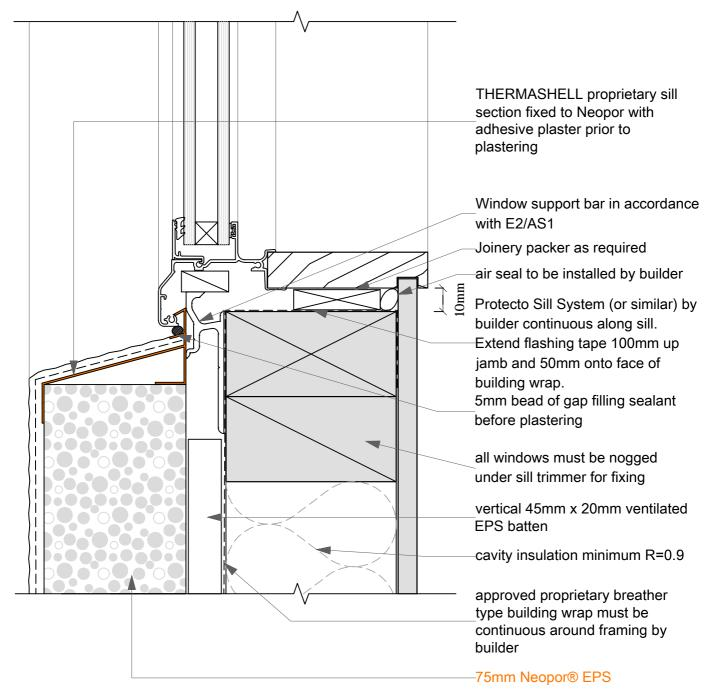
caution: to ensure the proprietary flashings for this system can be installed correctly, please allow a gap of 24mm from the surface of the building paper to the backside of the aluminium joinery
