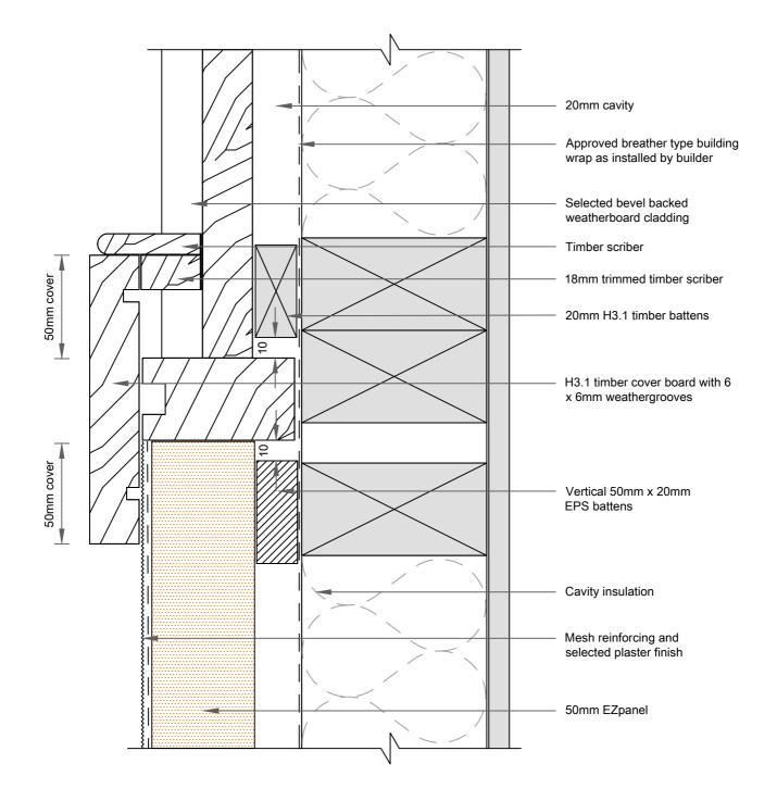
**18E** VERTICAL JOINT - WEATHERBOARD SCALE: 1:2 EZPANEL
