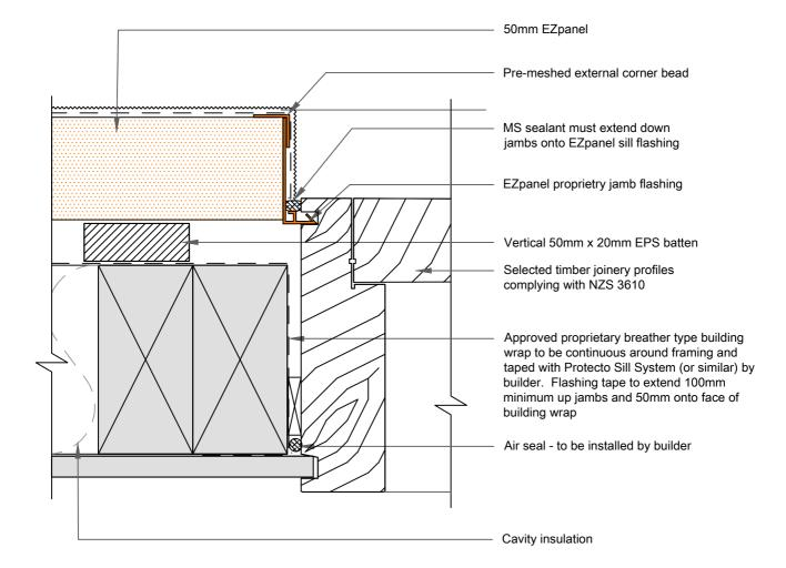
Note: Jambs and head flashing must be sealed or PVC welded where they intersect Caution:
