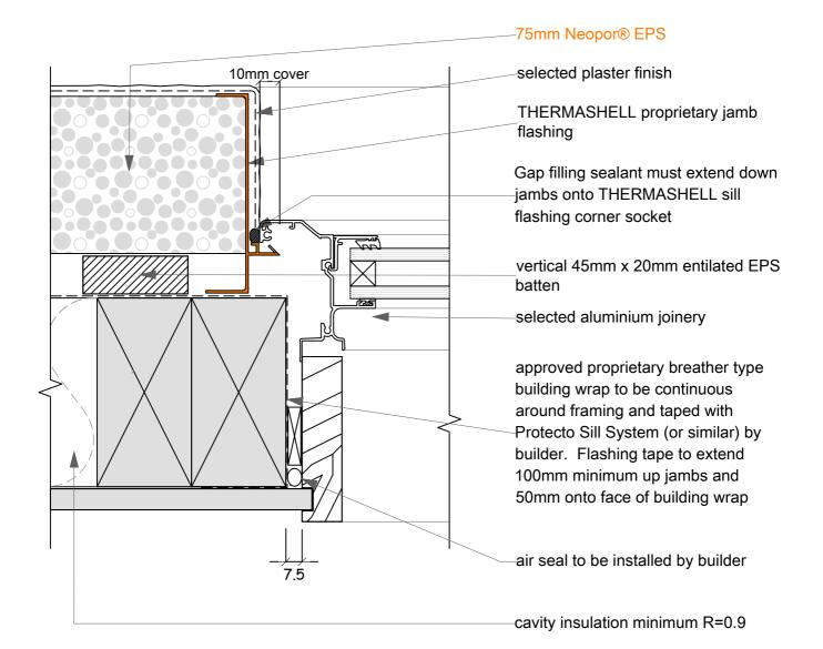
note: jambs and head flashing must be sealed or PVC welded where they intersect
