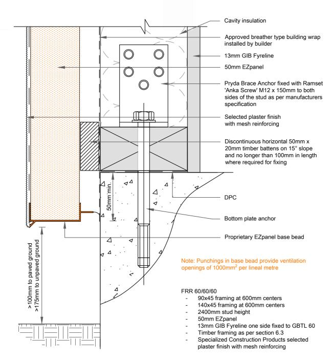
The external walls are required to be fire rated depending upon the situation when the wall is close to a boundary or a neighboring property in order to comply with NZBC clause C3. The walls included in this section are load bearing walls as per NZS 3604. Special attention must be paid to junctions and penetrations in external walls. The external claddings may be required to be fixed over a cavity and the cavity must not open into the roof space or sub floor space.
