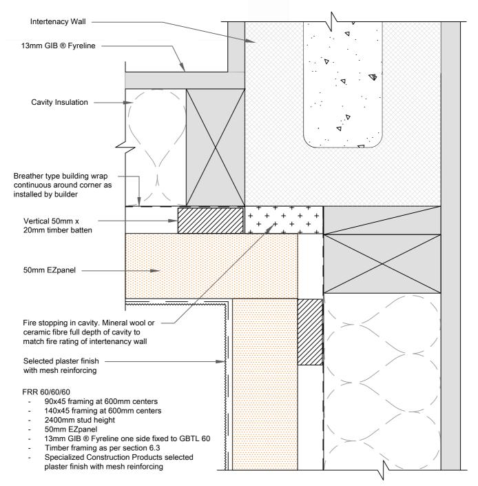
The external walls are required to be fire rated depending upon the situation when the wall is close to a boundary or a neighboring property in order to comply with NZBC clause C3. The walls included in this section are load bearing walls as per NZS 3604. Special attention must be paid to junctions and penetrations in external walls. The external claddings may be required to be fixed over a cavity and the cavity must not open into the roof space or sub floor space.
