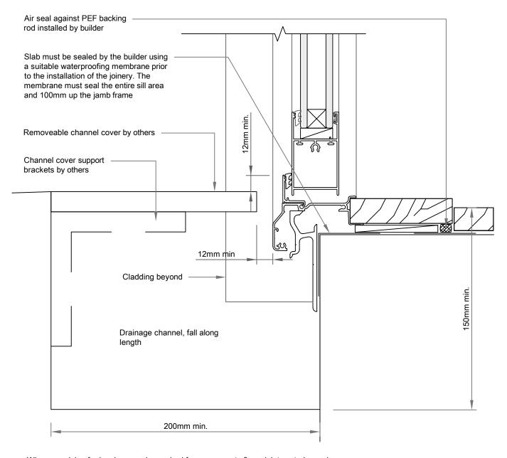
Where provision for level access is required from a concrete floor slab to exterior paving this shall be as shown in Figure 17B with:
