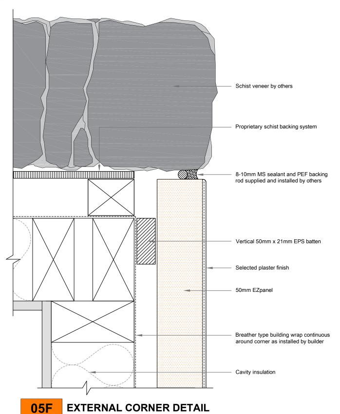
Schist - 50mm EZpanel - 20mm cavity with EPS Battens
