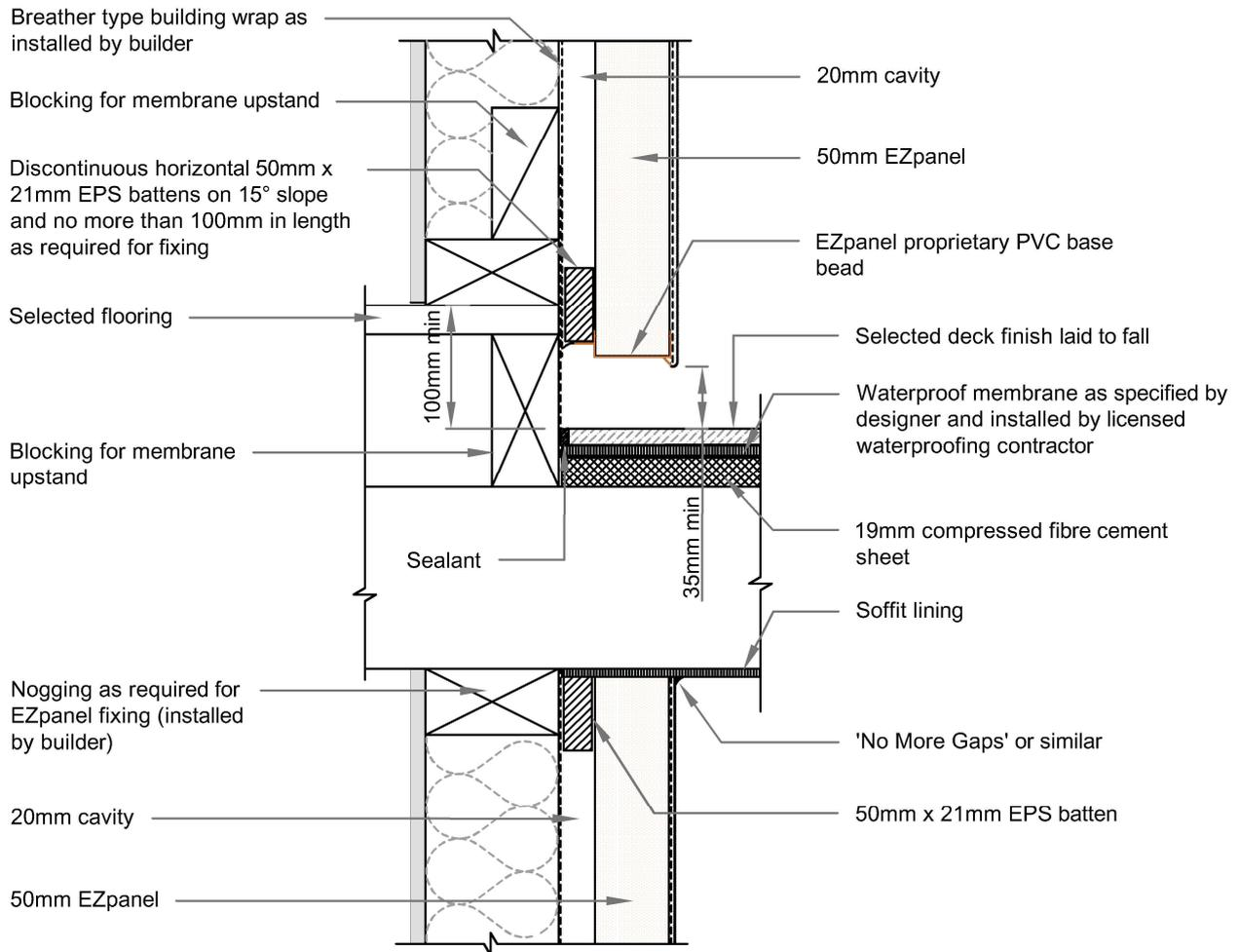
Note: Waterproof membrane must extend 200mm up vertical surface under approved building paper and a minimum of 150mm up behind the cladding system
