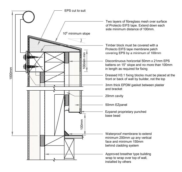
Note: If parapet wall top is wider than 300mm - it must have a minimum slope of 30°
