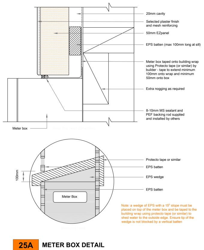
50mm EZpanel - 20mm cavity with EPS Battens
