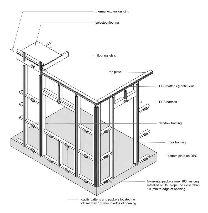
Note: For all wind zones EZpanel fixings to be at maximum 300mm centers to perimeter of panel edges and to intermediate studs.
