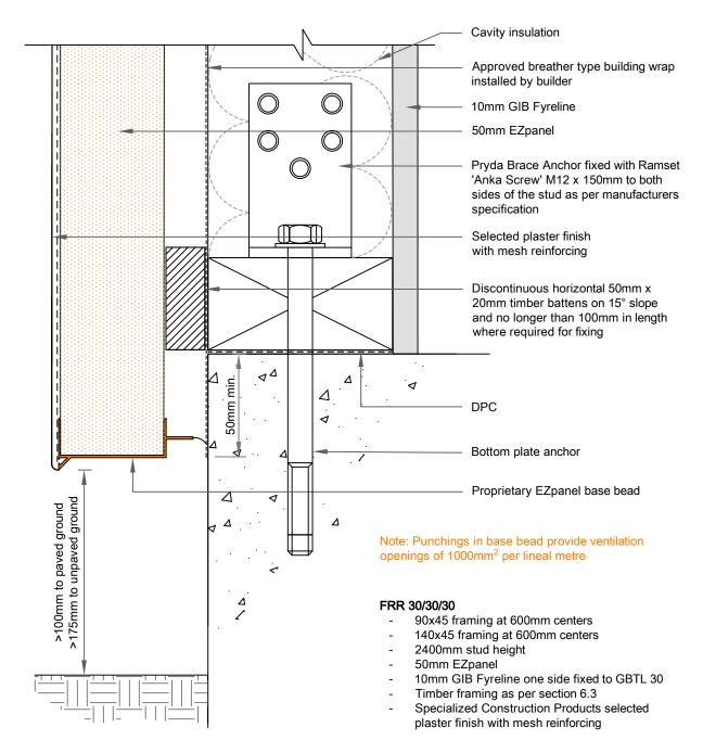
The external walls are required to be fire rated depending upon the situation when the wall is close to a boundary or a neighboring property in order to comply with NZBC clause C3. The walls included in this section are load bearing walls as per NZS 3604. Special attention must be paid to junctions and penetrations in external walls. The external claddings may be required to be fixed over a cavity and the cavity must not open into the roof space or sub floor space.
