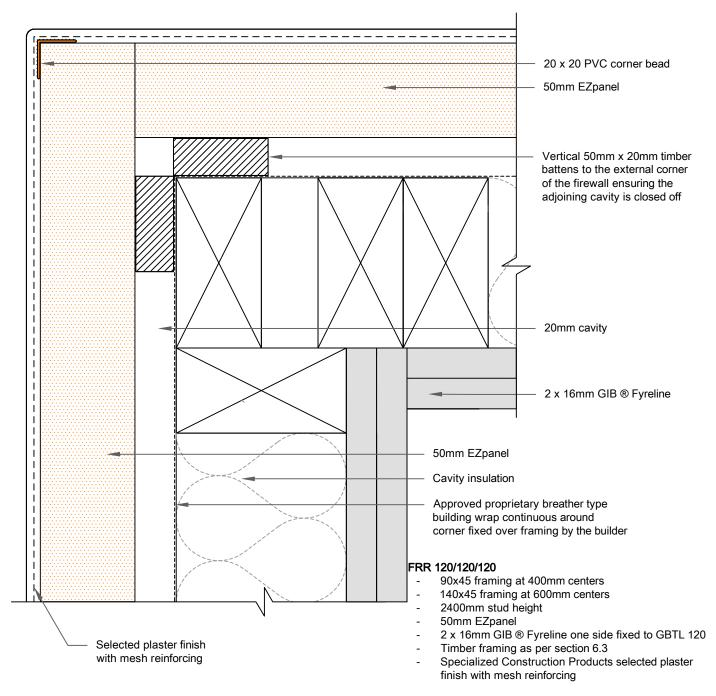
The external walls are required to be fire rated depending upon the situation when the wall is close to a boundary or a neighboring property in order to comply with NZBC clause C3. The walls included in this section are load bearing walls as per NZS 3604. Special attention must be paid to junctions and penetrations in external walls. The external claddings may be required to be fixed over a cavity and the cavity must not open into the roof space or sub floor space.
