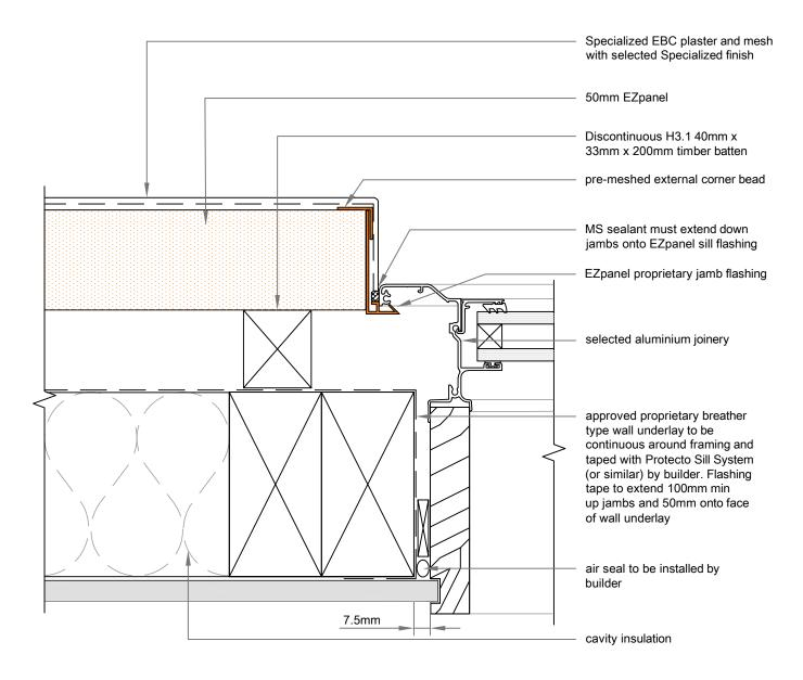
note: jambs and head flashing must be sealed or PVC welded where they intersect
