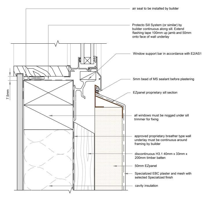
note: a 5° sloped sill trimmer must be used if the back of the glazing pocket is positioned back past the line of wall frame
