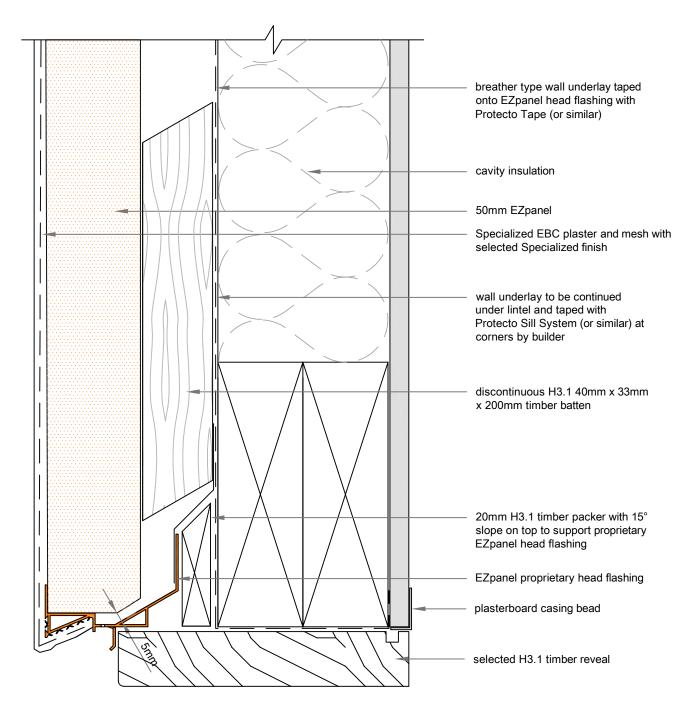
note: punchings in head flashing provide ventilation openings of 1000mm<sup>2</sup>per lineal metre
