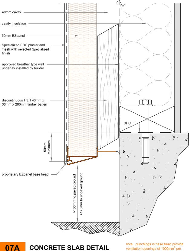
**CONCRETE SLAB DETAIL** 50mm EZpanel - 40mm cavity with timber battens SCALE: 1:2
