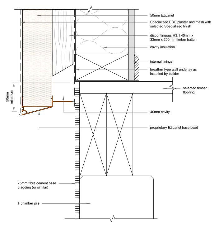
note: punchings in base bead provide ventilation openings of 1000mm<sup>2</sup> per lineal metre
