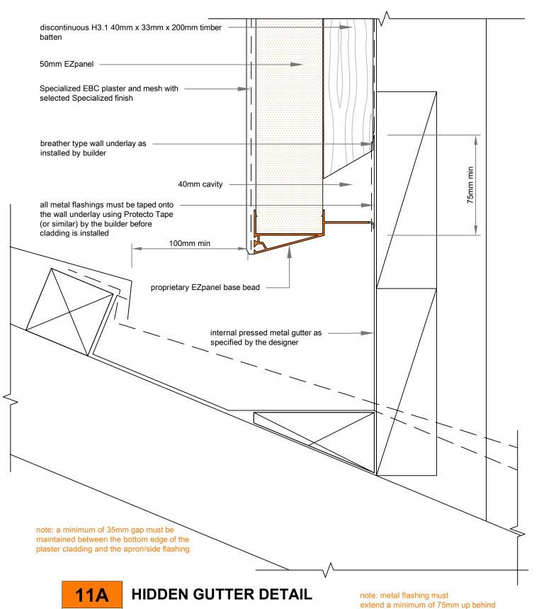
50mm EZpanel - 40mm cavity with timber battens
