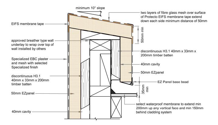
note: if roof is being used as an internal gutter the cladding must be a minimum of 100mm above the membrane surface
