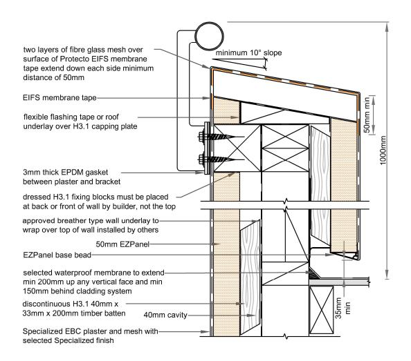
note: if parapet wall top is wider than 300mm - it must have a minimum slope of 30°
