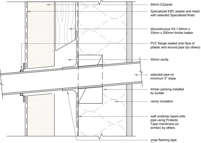
25mm around pipe and 100mm onto wall underlay
