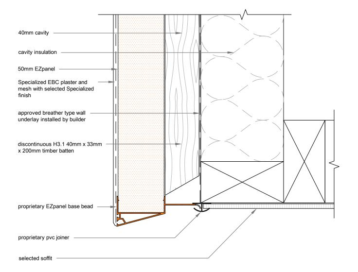
note: punchings in base bead provide ventilation openings of 1000mm<sup>2</sup> per lineal metre
