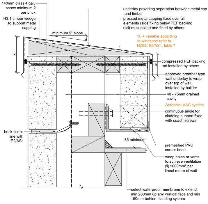
note: if roof is being used as an internal gutter the cladding must be a minimum of 100mm above the membrane surface
