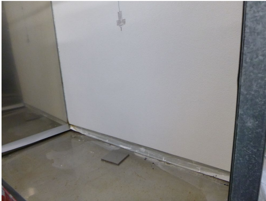
Figure 3: Rear of heat rain wall after 240 cycles
