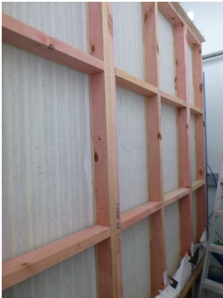
Figure 3: Rear of heat rain wall after 240 cycles
